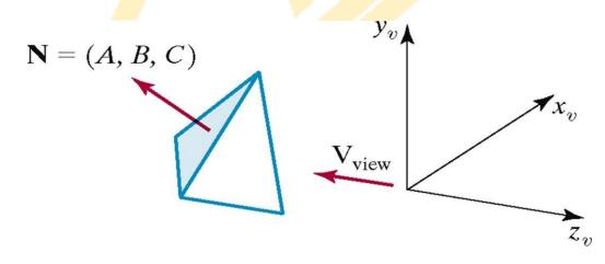
•  $V_{\text{view}}$  is a vector in the viewing direction from the eye ("camera") position, a polygon surface is a back face if:
