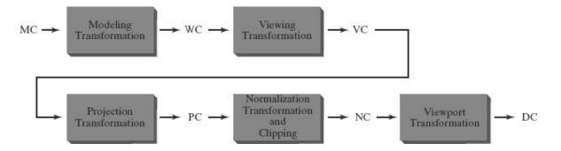
Figure above shows the general processing steps for creating and transforming a three dimensional scene to device coordinates.
