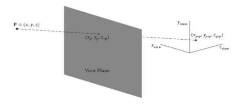
The projection line intersects the view plane at the coordinate position ( $x_p$ ,  $y_p$ ,  $z_{vp}$ ), where  $z_{vp}$  is some selected position for the view plane on the  $z_{view}$  axis.
