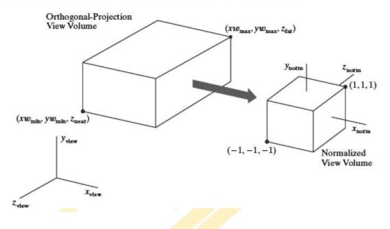
The normalization transformation for the orthogonal view volume is
