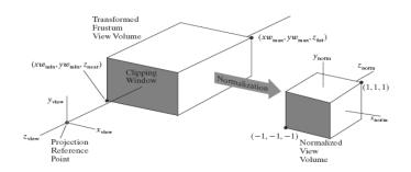
Because the centerline of the rectangular parallelepiped view volume is now the  $z_{view}$  axis, no translation is needed in the *x* and *y* normalization transformations: We require only the *x* and *y* scaling parameters relative to the coordinate origin.
