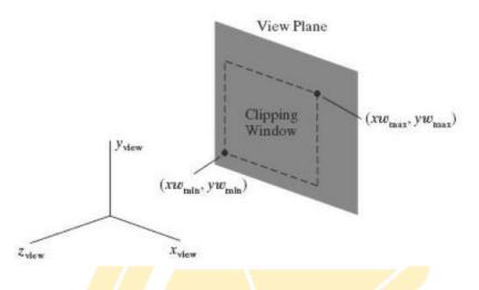
Because projection lines are perpendicular to the view plane, these four boundaries are planes that are also perpendicular to the view plane and that pass through the edges of the clipping window to form an infinite clipping region, as in Figure below.
