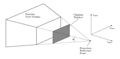
For a given projection reference point and view-plane position, the field-of view angle determines the height of the clipping window from the right triangles in the diagram of Figure below,
