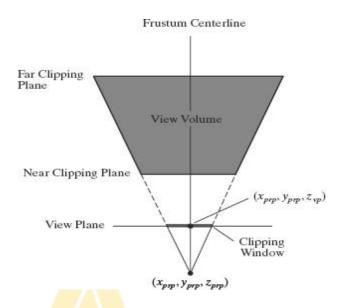
Because the frustum centerline intersects the view plane at the coordinate location ( $x_{prp}$ ,  $y_{prp}$ ,  $z_{vp}$ ), we can express the corner positions for the clipping window in terms of the window dimensions:
